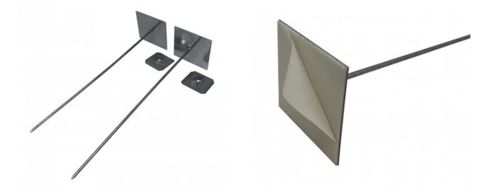
Self-Adhesive Base Hangers are designed to efficiently fix insulation to metal, attenuators, enclosures and smooth sound substrates. Surfaces must be clean, dry and free of dust, grease, oil and any other loose matter before the Hangers are applied. It is recommended that the user make test bonds to ensure the compatibility between the substrate and adhesive.
