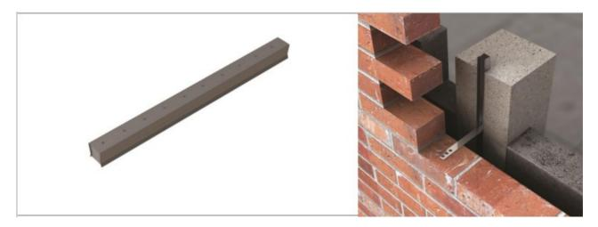
Cast in dovetail slot, available in stainless steel or pre-galvanised steel. These systems are pre-filled with polystyrene to prevent concrete ingress.
