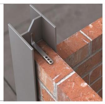
Frame cramp (supplied in stainless to BS EN 10088-1.4301) for restraining masonry to new or existing structures and for building in non-structural elements (frames etc). Supplied with a slot in upstand to allow various fixings.
